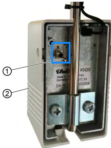
Fig. 45: Assigning a function to the knee button
