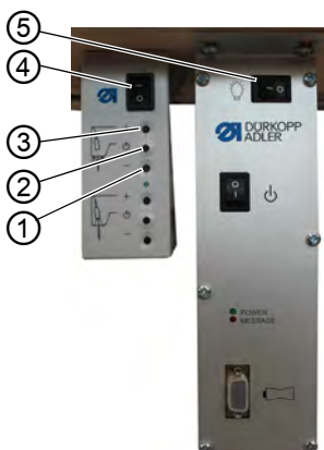
Fig. 39: Switching on and off the sewing lamp
